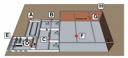
Initially, the assumption is that eight base station (shown as red circles) should be adequate as measurement is not done at this point.
