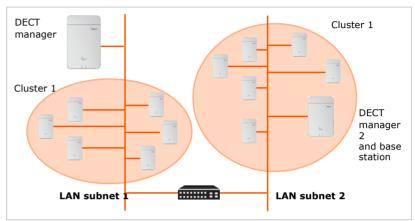
In installations with multiple DECT managers, handover and roaming between base stations of different DECT managers are possible when the clusters are synchronised. Load balancing is not possible.
