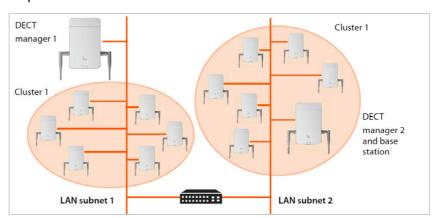
In installations with multiple DECT managers, handover and roaming between base stations of different DECT managers are possible when the clusters are synchronised.
