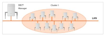
The DECT manager is connected to the base stations and the PABX via the local network and is therefore not dependent on DECT ranges. Base stations that are far apart can be grouped into different clusters if synchronisation is barely, or not, possible, and is not required. All the base stations of a DECT manager must belong to the same LAN subnet of the DECT manager.
