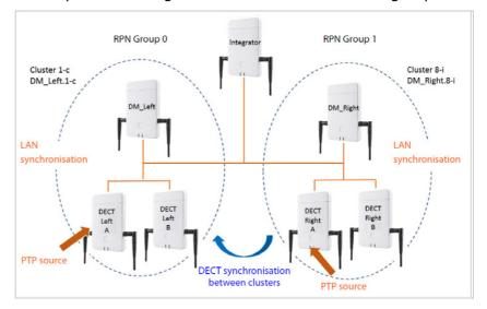
There are a number of conditions to be considered when setting up a DECT network. They affect the subscribers' requirements for the telephone system as well as the technical requirements for the DECT wireless network. These conditions must therefore be recorded and evaluated
