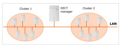
For installations in different LAN subnets, multiple DECT managers with one DECT manager per subnet are required. The DECT manager function can be installed in parallel on the same device (depending on the capacity of the local base station). Multiple DECT managers are also required when the requirement is to connect more than 250 handsets or provide more than 60 connection channels.
